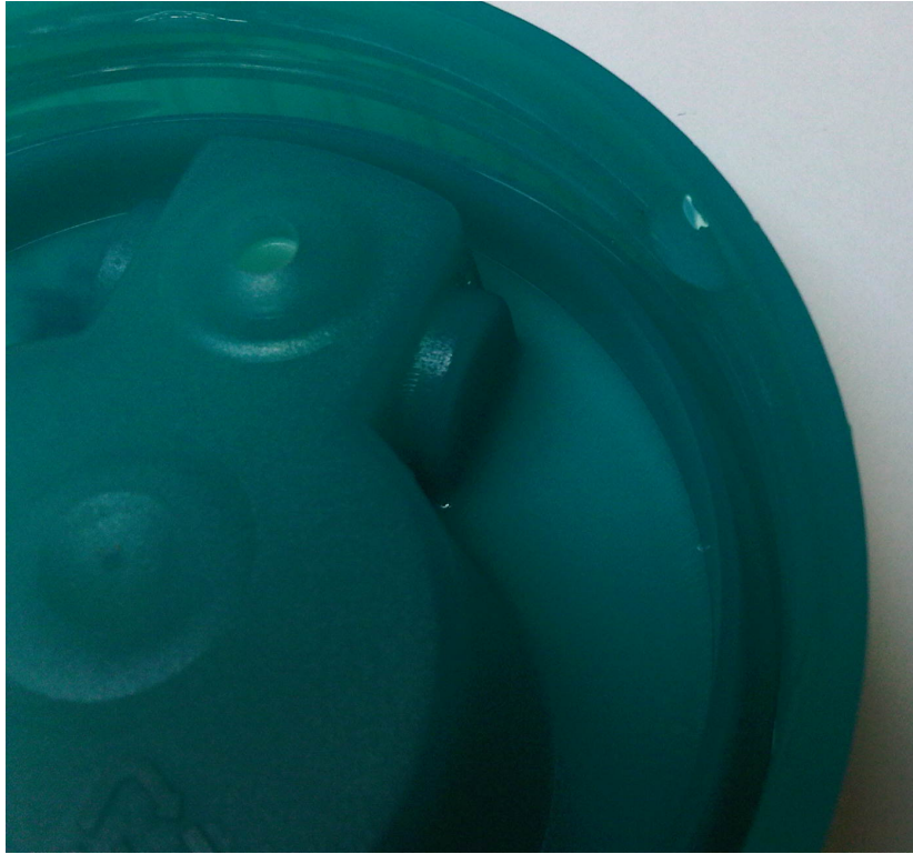
Figure 8: Liquid found in the cap thread of one bottle after leak testing.
